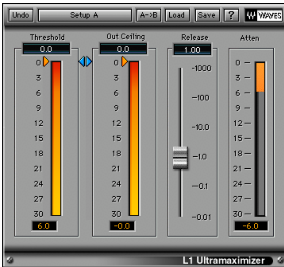
Uncontrollable overload of a dynamic plug-in that lacks an input attenuation option
